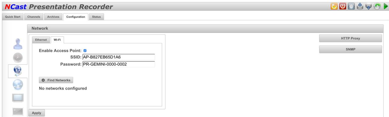
The Presentation Recorders can function as either a WiFi client or an Access Point. The default Access Point name is “AP-” followed by the units MAC address. The default password is the unit's serial number, found on the outside of the case. Uncheck the Access Point checkbox to configure the unit as a WiFi client.
