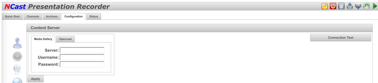
Entering the server address and credentials will allow the recorder to automatically upload and stream to the Media Gallery.
