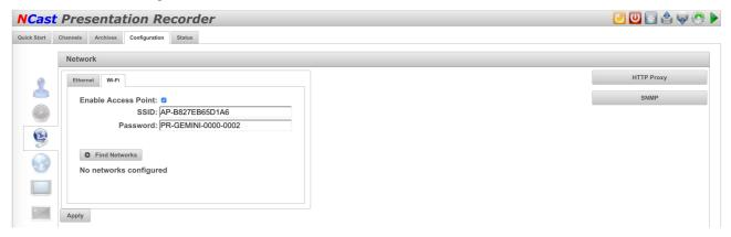
The Presentation Recorders can function as either a WiFi client or an Access Point. The default Access Point name is "AP-" followed by the units MAC address. The default password is the unit's serial number, found on the outside of the case. Uncheck the Access Point checkbox to configure the unit as a WiFi client.
