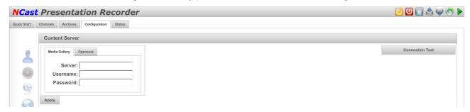
Entering the server address and credentials will allow the recorder to automatically upload and stream to the Media Galllery.
