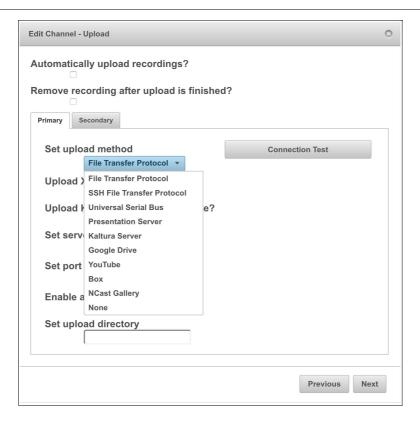
There is a Primary Upload choice and a Secondary Upload choice. This allows the Presentation Recorder to target two different entities for delivery of the file.
