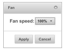
The recorder does not adjust the fan speed automatically. A user can read the CPU temperature (on the Status tab) and adjust fan speed according to the cooling needed. The minimum value is 30%. A value of 100% should be used if the unit is in a rack with other equipment.
