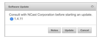
If the encoder is not on the latest release, select the desired revision and click "Update". All necessary update files will be downloaded over the net and the encoder will reboot once the new firmware has been installed.
