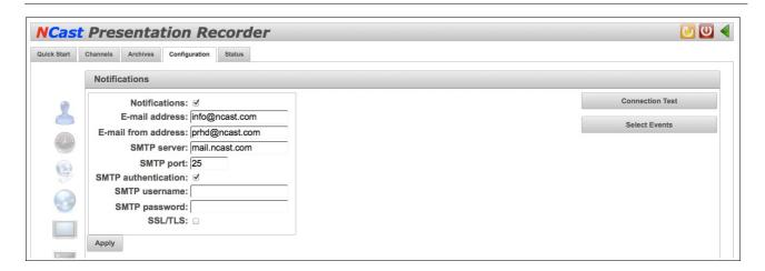
Event are categorized by their severity level (Info, Warning, Error and Critical), and by their specific action or type (e.g. Session start, Recording start, etc.). Events can be system-wide (e-mails are sent to the system administrator) or Channel specific (a subset of events is associated with a single Channel and sent to an e-mail address associated with that Channel).
