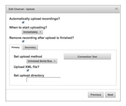
Due to the wide variety (and often poor performance) of USB sticks, all archive files are first recorded and finished on the internal storage of the unit and then transferred to the external USB drive.
