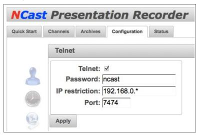
If the interface is enabled, secure the interface with a unique and non-dictionary password, and configure the IP restriction field to only allow the IP address of the controller unit to command the Presentation Recorder.
